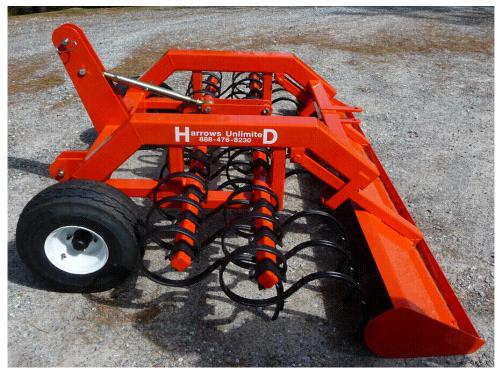
The JD Special is John Dienhart's original harrow design. A single tire mounting hole now provides the operator assurance that the harrow frame will be in correct level operating position before adjustments are made within the arena.
